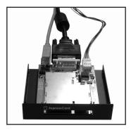
2. Remove the cover from a 3.5" drive bay, on the front panel of the host computer case, then feed the remaining ends of the cables used in step #1 through the open bay:
